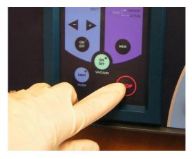
D) The key **STOP** can be used in case of errors to activate the EMERGENCY-OFF for the pressure generation.
