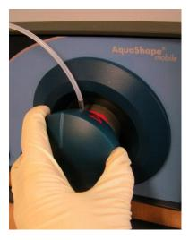
B) Remove the sealing cap.
