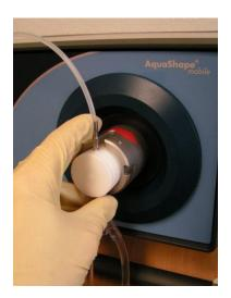
D) Clamp the liquid delivery tubes and cut off the delivery system above the pressure container.
