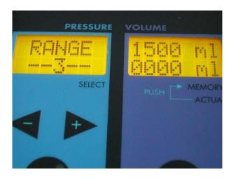
In order to activate this display it is necessary to press the MEM button prior to the operation.
