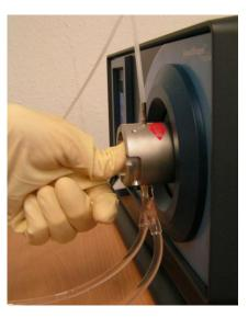
CAUTION: If the pressure container is not correctly engaged, it is not possible to build-up pressure
