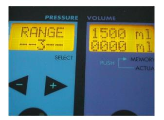
This procedure may be repeated as often as required. The right-hand upper display then indicates the total liquid consumption whereas the right-hand lower display always shows the amount of liquid used during the current suction sequence.
