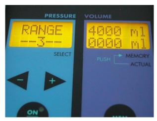
By pressing the MEM button for three seconds all consumption displays are reset to ZERO.
