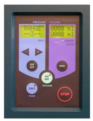
C) Select the pressure range ( RANGE 1 to 5 ) using the  $\pm$ - buttons.
