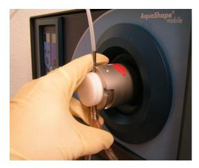
Remove the sealing cap from the pressure container socket by turning it in the anticlockwise direction. Insert the pressure container in the socket provided.
