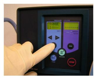
B) The pressure generation unit is activated by pressing the ON/OFF switch on the PRESSURE control panel
