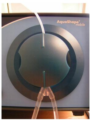
If the surface markings of the closing cap are arranged as shown in the picture, the cap is attached in the correct position.
