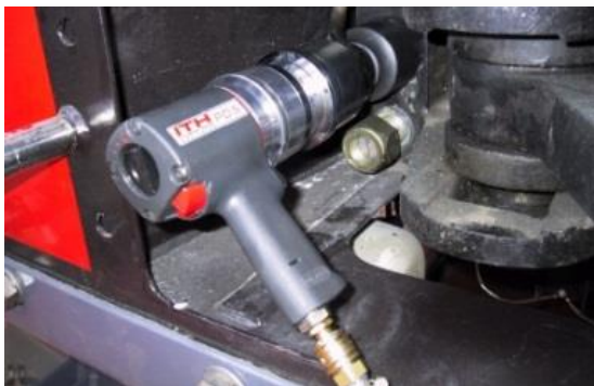
This clutch bolt connection M36 (1 3/8'') of a tractor unit is tightened with a PDS 250.
