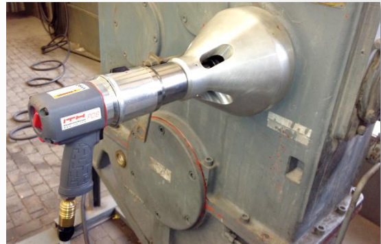
Customer specific supports (reaction arms) can be delivered for all ITH Nut Runners. This conical support was used to tighten the bolts of a waste incineration machine with a ITH PDS 250.
